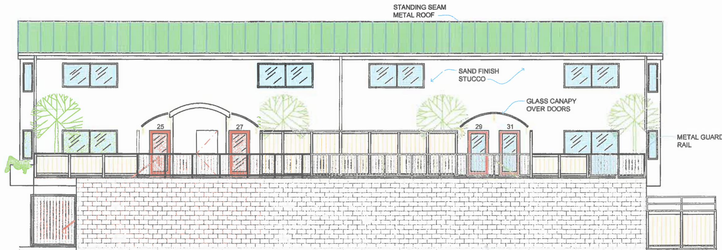
NATURAL GRAY CONC. BLOCK MASONRY WALLS 8x8x16 STAGG., RODDED JOINTS
